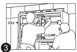
Place the next cabinet into position using the T-brace. Use C-clamps to clamp the stiles of the 2 cabinets together and countersink two 2 ½" wood screws into the stiles. Make sure the cabinet is level and plumb. Using 3" screws, screw the cabinet to the wall through the mounting rails and into the studs. Repeat the steps with the remaining wall cabinets. Make sure they are level, plumb and that all screws have been tightened.
