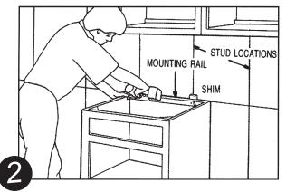
Drill pilot holes through the mounting rails at the stud locations you have marked. Then drive wood screws in leaving them loose enough to allow for adjustment. After making sure the cabinet is still level and plumb, fasten the top and bottom screws securely.
