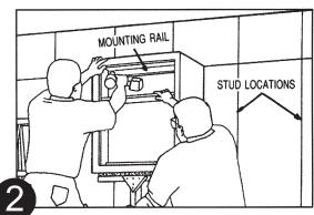
Drill pilot holes through the mounting rails at the stud locations you have marked. Then drive wood screws leaving them loose enough to allow for adjustment. Next, use a level to see if the cabinet front is plumb (vertically level). If it is not, you can use shims to bring the cabinet into plumb. After making sure the cabinet is level and plumb, fasten the top and bottom screws securely.
