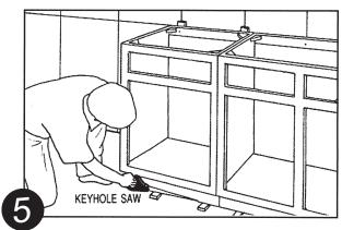
After all cabinets are in place, make sure they are still level and plumb. If necessary adjust your shims then make sure all mounting screws have been tightened. At this point use your keyhole saw to trim the shims even with your cabinet.
