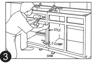
Place the next cabinet into position and level it so that it lines up with the first cabinet and your guidelines marked on the wall. Use C-clamps to clamp the stiles of the 2 cabinets together and countersink two 2 ½" wood screws into the stiles. Make sure the cabinet is level and plumb as you did before. Then screw the cabinet to the wall through the mounting rails and into the studs. Repeat these steps with the remaining base cabinets.
