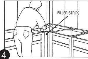
If you are not using a special corner cabinet, use filler strips at the corner to allow enough space for doors and drawers to operate smoothly. Join the filler strips in the same as you do the stiles of the cabinets. To support counter top, attach 1" x 2" wood strips to the wall along your guidelines so they are level with your cabinets. For instructions on using corner cabinets, see the notes section of this brochure.
